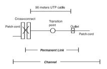
Two link configurations are defined for testing purposes. The permanent link includes the horizontal distribution cable, telecommunications outlet/connector or transition point and one horizontal cross-connect component including the mated connections. This is assumed to be the permanent part of a link. The channel is comprised of the permanent link plus cross-connect equipment, user equipment cord and cross-connect patch cable.
