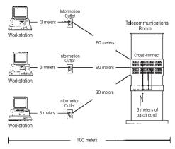
In addition to the 90 m of horizontal cable, a total of 10 m is allowed for work area and telecommunications room patch and jumper cables.
